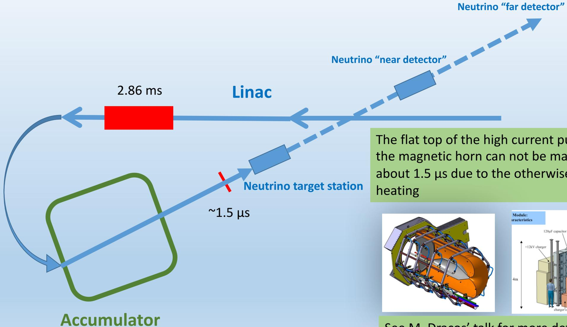
The flat top of the high current pulse of 350 kA in the magnetic horn can not be made longer than about  $1.5 \mu\text{s}$  due to the otherwise excessive ohmic heating
