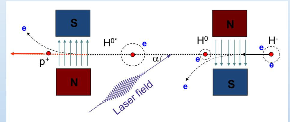
Lorentz stripping of the first electron by a dipole magnet in the first step, resonant excitation of the second electron by the laser in the second step, and, finally, stripping of the excited electron by the second dipole magnet
