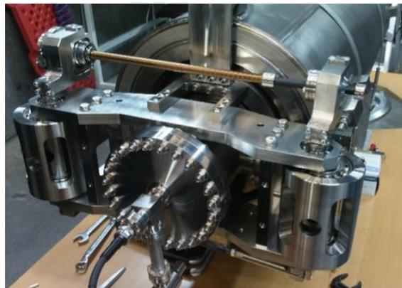
Assembly and adjustment of the cold tuning systems
