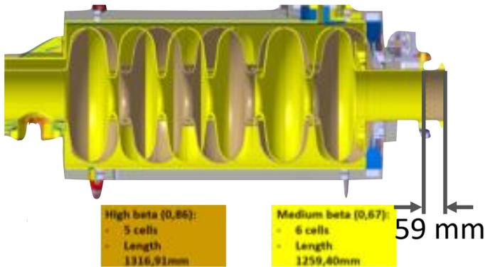
ESS elliptical cryomodule with four 6-cell cavities and four power couplers for up to ~1.1 MW peak RF power.
