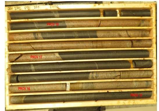
Drill cores from the granite rock
