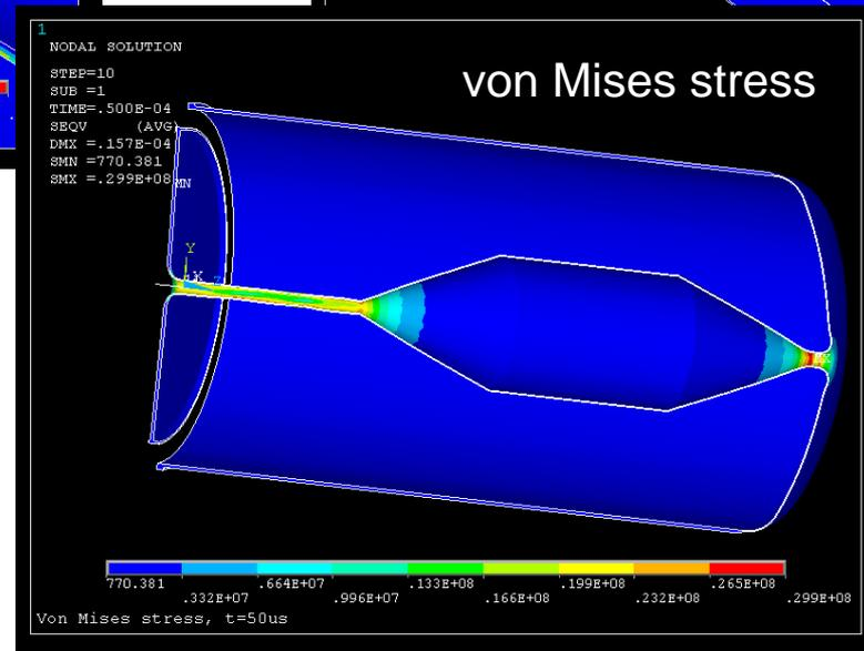
Maksimum von Mises stress is about 30 MPa. Stress is higher under a sequence of current pulses.
