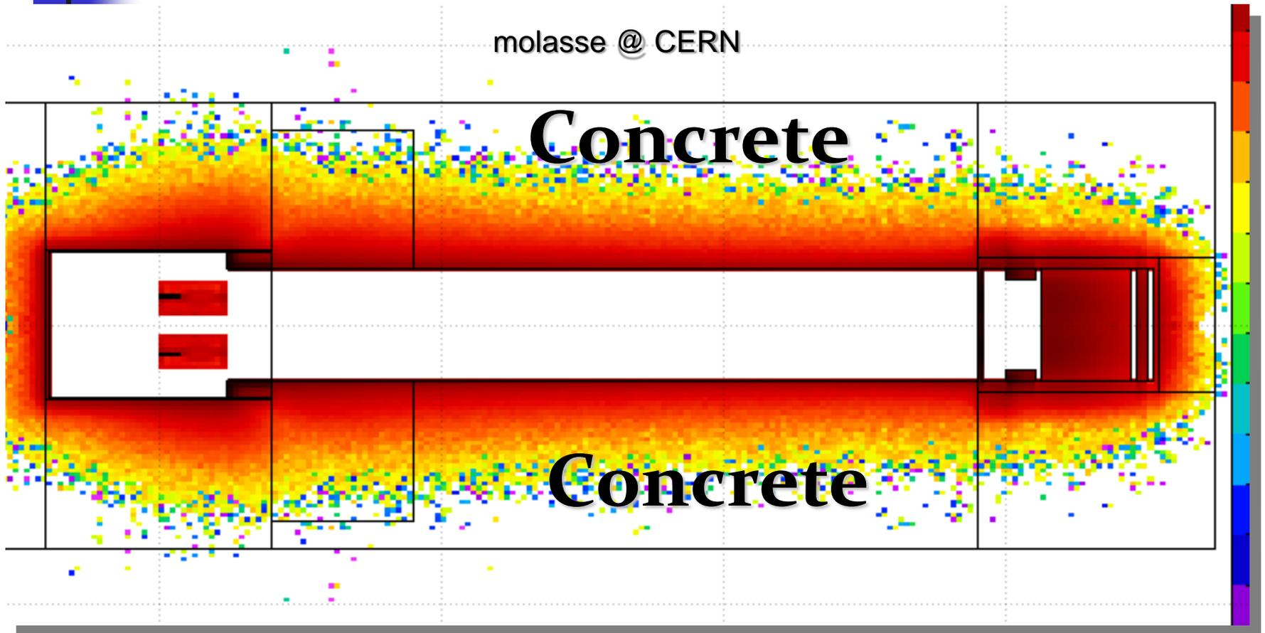
A 6m thickness concrete wall surrounding all the layout limits the production of radionuclides in the molasse. Especially, the production of  $^{22}\text{Na}$  and tritium could represent a negative impact by contaminating the ground water.
