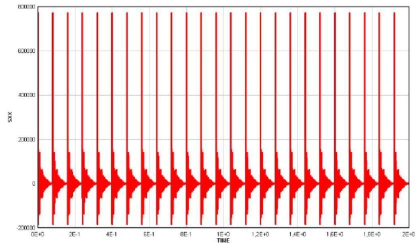
Such results can be used to estimate the fatigue life of the horn
