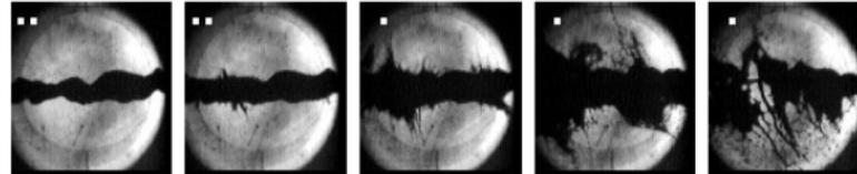
MERIT experiment: Beam-induced splashing of mercury jet (c.200 J/cc)
