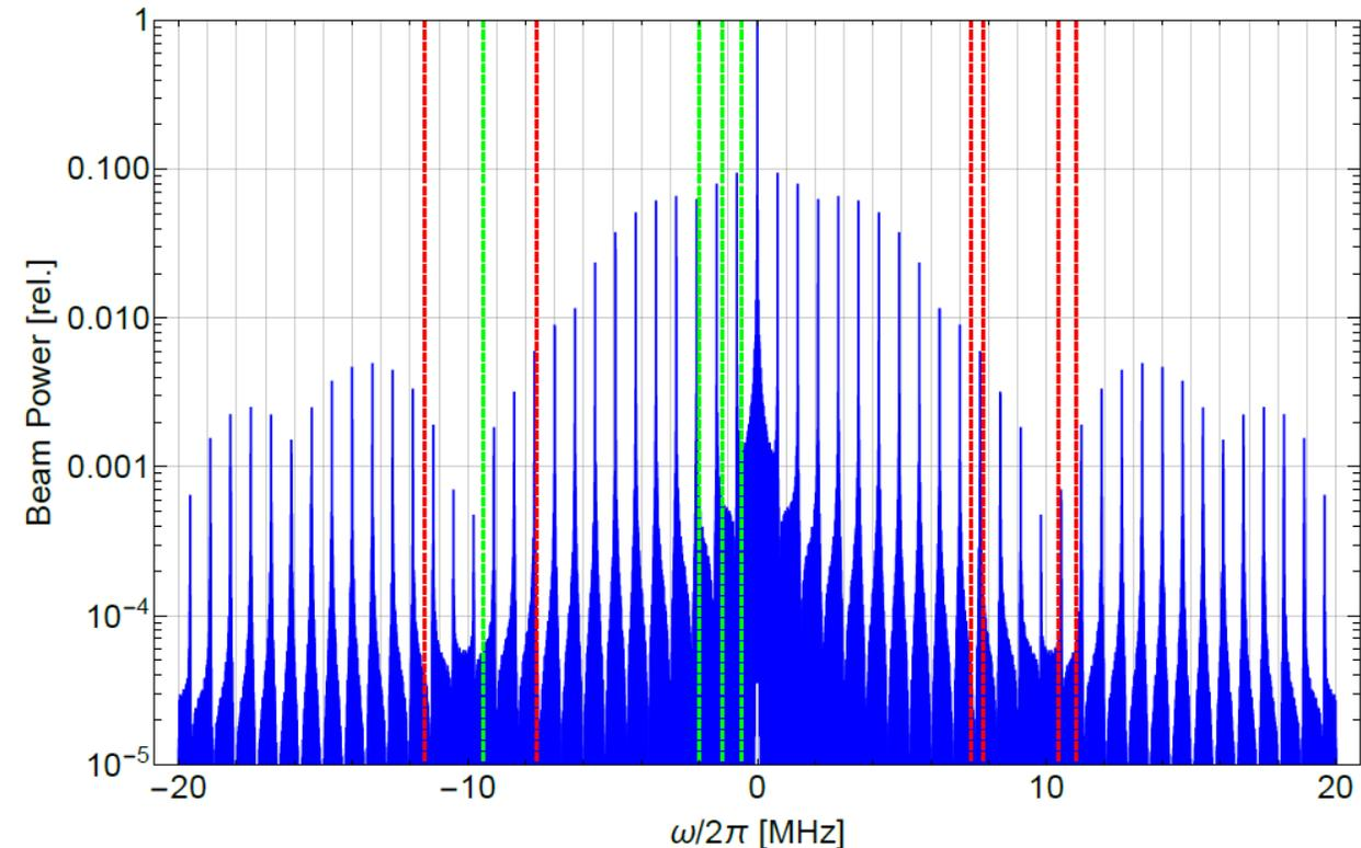
Center frequency 352 MHz, RF bunching frequency, HOMs are shown in red and the modes in the accelerating passbands in green.
