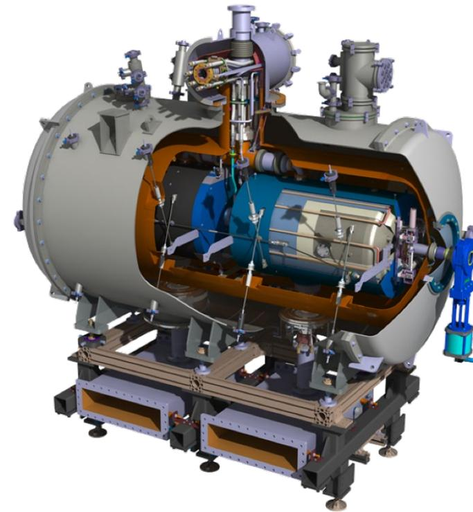
ESS Spoke cryomodule with two double spoke cavities, and two power couplers
