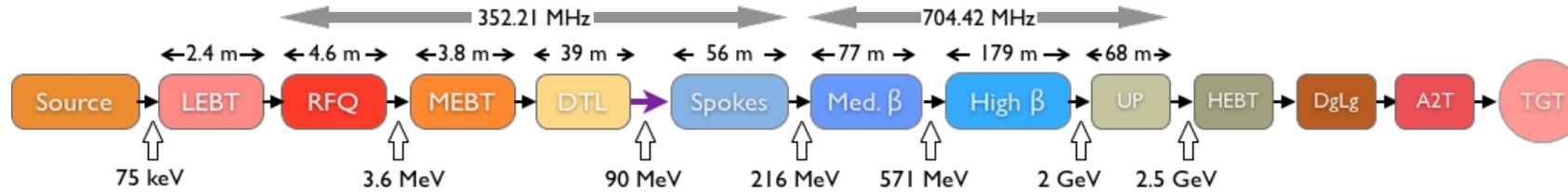
The accelerator layout, with normal conducting section and superconducting section. Indicated is the energy upgrade to 2.5 GeV.
