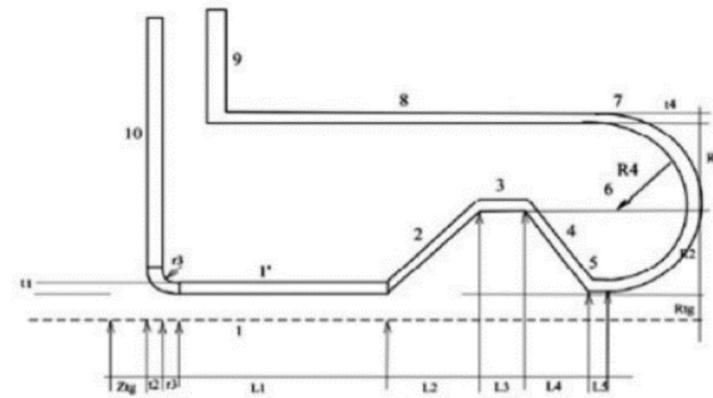
Horn parametrization based on Genetic Algorithm
