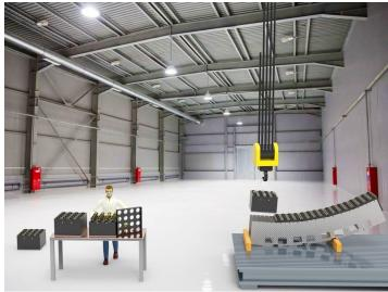
(b) Illustration of the assembly of two PMT mounting boxes by a technician, as well as the mounting of six photo-module boxes into an arch for subsequent mounting on the detector frame (see Fig. 5.7)
