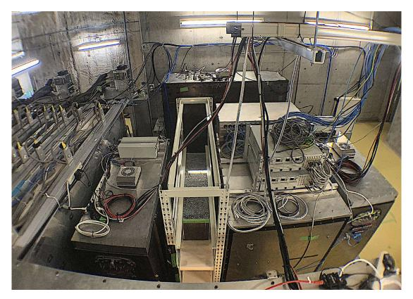
Figure 5.43: A NINJA detector includes 9 water-target ECC elements. The NINJA detector is in the centre of the figure. The white rack consists of three tiers, with 3 ECC elements on each tier, for a total of 9 ECC elements in operation. An emulsion shifter and a scintillation tracker, which add timing information to emulsion tracks, are placed downstream from the ECC elements for  $\mu$  identification (by connecting to the Baby-MIND, which is one of the T2K near detectors).
