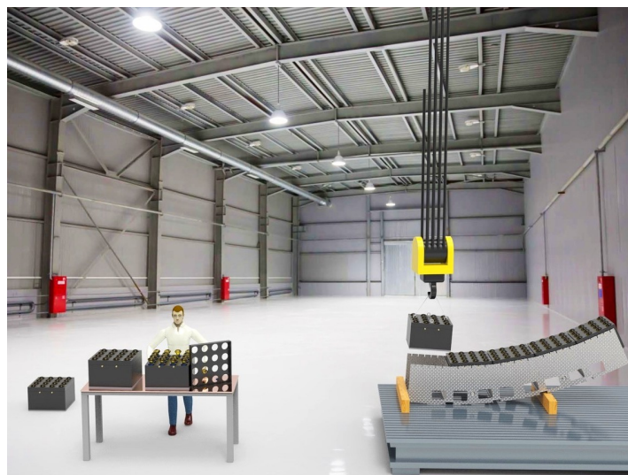
(b) Illustration of the assembly of two PMT mounting boxes by a technician, as well as the mounting of six photo-module boxes into an arch for subsequent mounting on the detector frame (see Fig. 6.7)
