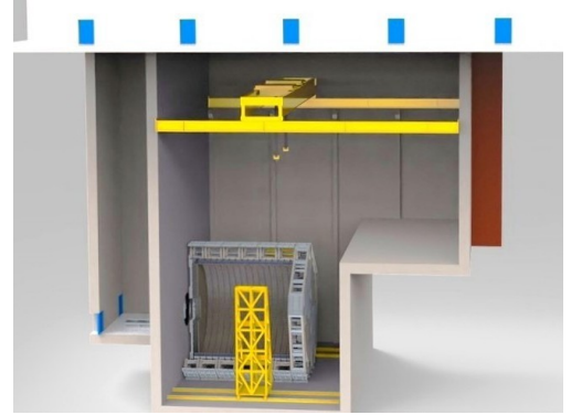
(b) An artistic rendering of the near-detector cavern, including the water Cherenkov component in the mounting phase.
