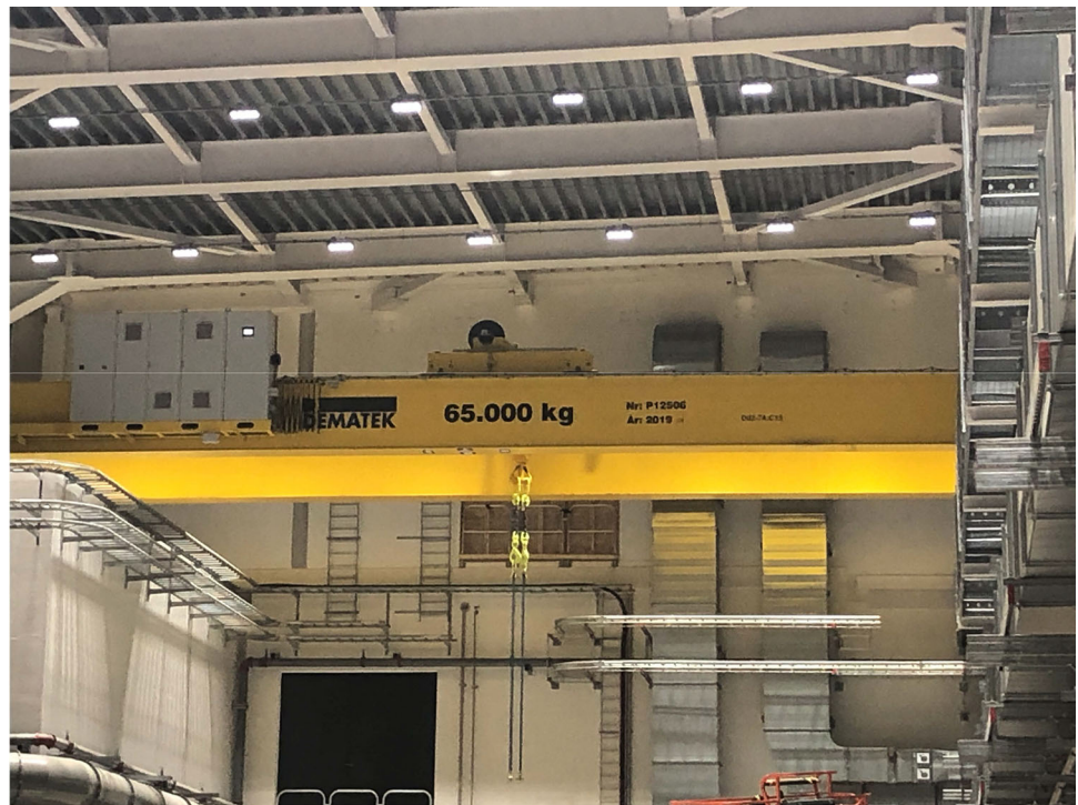
Fig. 207 Largest existing ESS overhead crane currently in operation in the D02 Target building
