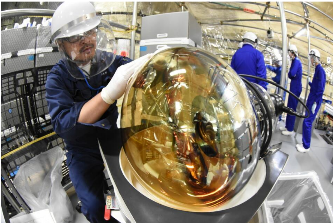
One of the photo-detectors at the Super-Kamiokande. Kamioka Observatory, ICRR (Institute for Cosmic Ray Research), The University of Tokyo
